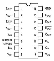
Pin assignment is for Dual–in–Line Package. For PLCC pin assignment, see Table 1.
