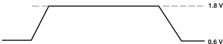
Figure 9. 'LC31 Input Levels
