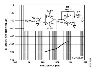
Figure 52. Channel Separation
