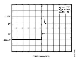
Figure 45. Negative Overload Recovery Time
