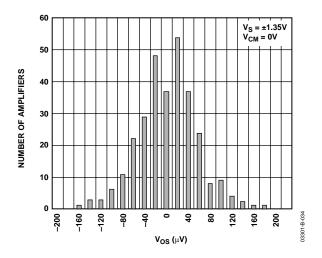
Figure 34. Input Offset Voltage Distribution
