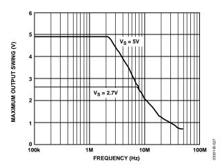
Figure 27. Maximum Output Swing vs. Frequency
