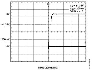
Figure 46. Positive Overload Recovery Time
