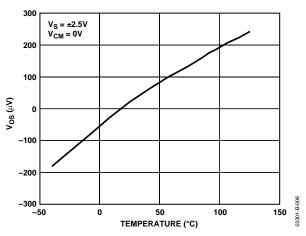
Figure 6. Input Offset Voltage vs. Temperature
