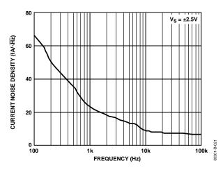
Figure 21. Current Noise Density vs. Frequency
