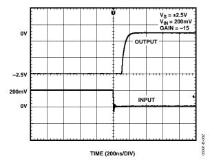
Figure 32. Positive Overload Recovery Time
