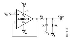
Figure 55. Driving Large Capacitive Loads
