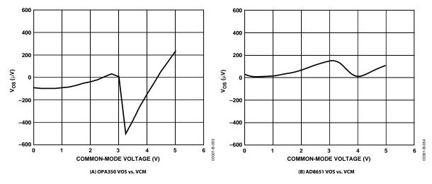
Figure 53. Input Offset Distribution over Common-Mode Voltage
