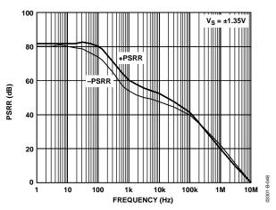
Figure 48. PSRR vs. Frequency
