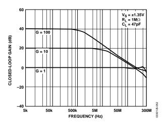
Figure 51. Closed-Loop Gain vs. Frequency
