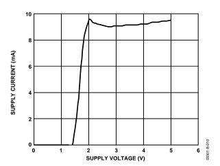
Figure 10. Supply Current vs. Supply Voltage
