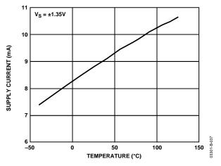
Figure 37. Supply Current vs. Temperature
