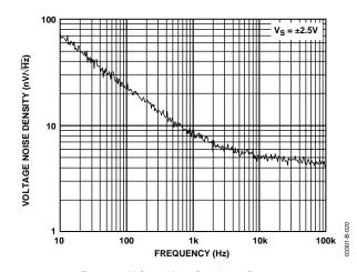
Figure 20. Voltage Noise Density vs. Frequency
