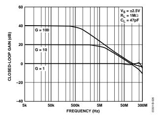
Figure 26. Closed-Loop Gain vs. Frequency
