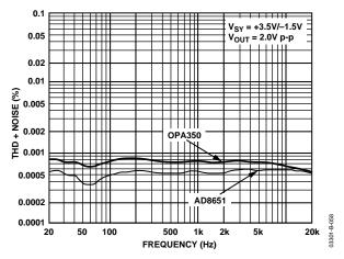
Figure 57. Total Harmonic Distortion
