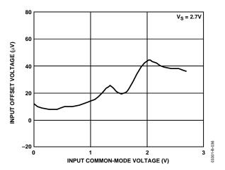
Figure 36. Input Offset Voltage vs. Common-Mode Voltage
