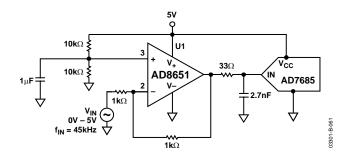
Figure 60. AD8651 Driving a 16-Bit ADC
