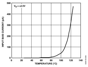
Figure 9. Input Bias Current vs. Temperature
