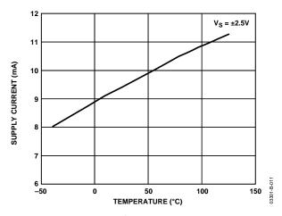
Figure 11. Supply Current vs. Temperature
