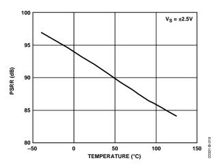
Figure 19. PSRR vs. Temperature
