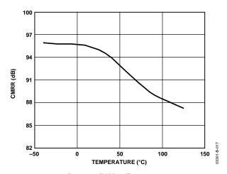
Figure 17. CMRR vs. Temperature
