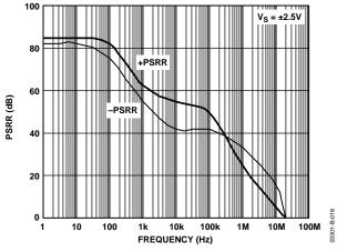
Figure 18. PSRR vs. Frequency
