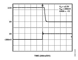
Figure 31. Negative Overload Recovery Time
