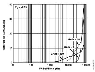
Figure 33. Output Impedance vs. Frequency
