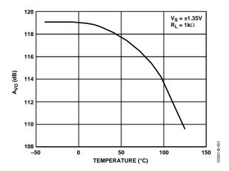
Figure 50. Open-Loop Gain vs. Temperature
