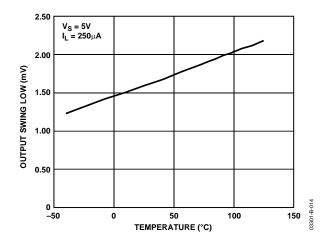
Figure 14. Output Voltage Swing Low vs. Temperature
