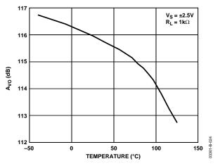
Figure 24. Open-Loop Gain vs. Temperature
