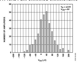
Figure 5. Input Offset Voltage Distribution
