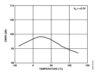
Figure 16. CMRR vs. Temperature
