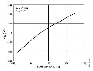
Figure 35. Input Offset Voltage vs. Temperature
