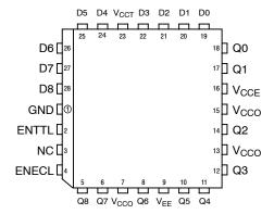
Figure 1. Pinout: PLCC-28 (Top View)
