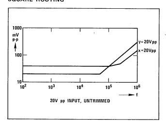
MULTIPLIER FEEDTHROUGH AT 20V p'-p INPUT, UNTRIMMED
