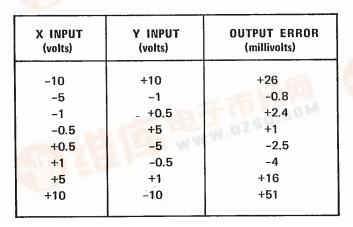
TYPICAL OUTPUT ERROR (mV) vs X AND Y INPUT VOLTAGE
