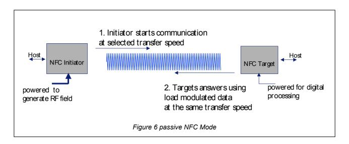
The PN531's firmware and contactless UART handle the NFC protocol.
