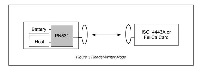
In the reader/ writer mode the PN531 enables communication to a passive ISO14443A/MIFARE<sup>®</sup> or FeliCa<sup>™</sup> card.
