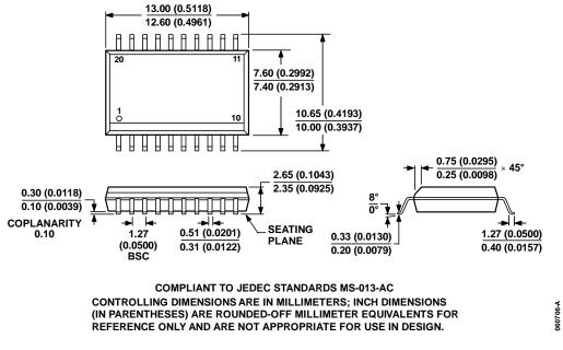
Figure 5. 20-Lead Standard Small Outline Package. Dimensions shown in millimeters and (inches).
