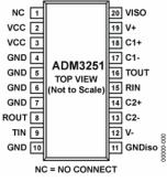
Figure 2. ADM3251E Pin Configuration
