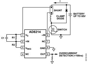
Figure 31. High Side Overcurrent Protection
