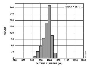
Figure 26. Output Current Distribution
