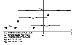
Figure 29. Hysteresis and Input Offset Voltage Definition
