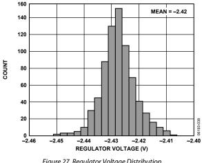
Figure 27. Regulator Voltage Distribution (With Respect to Vs)
