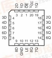
To ensure the high-impedance state during power up or power down, OE should be tied to V<sub>CC</sub> through a pullup resistor; the minimum value of the resistor is determined by the current-sinking capability of the driver.
