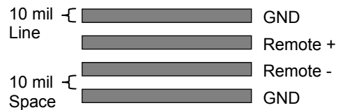
Figure 13 Recommended Remote Diode Circuit Board Interconnect
