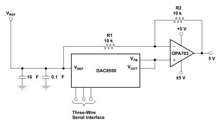
Figure 56. Bipolar Output Range
