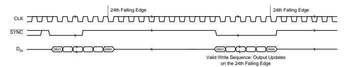
Figure 50. SYNC Interrupt Facility
