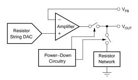
Figure 51. Output Stage During Power-Down
