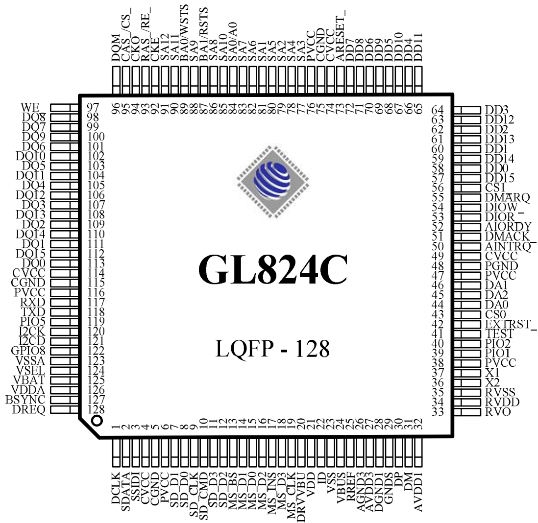
Figure 3.2 – 128 Pin LQFP Pinout Diagram
