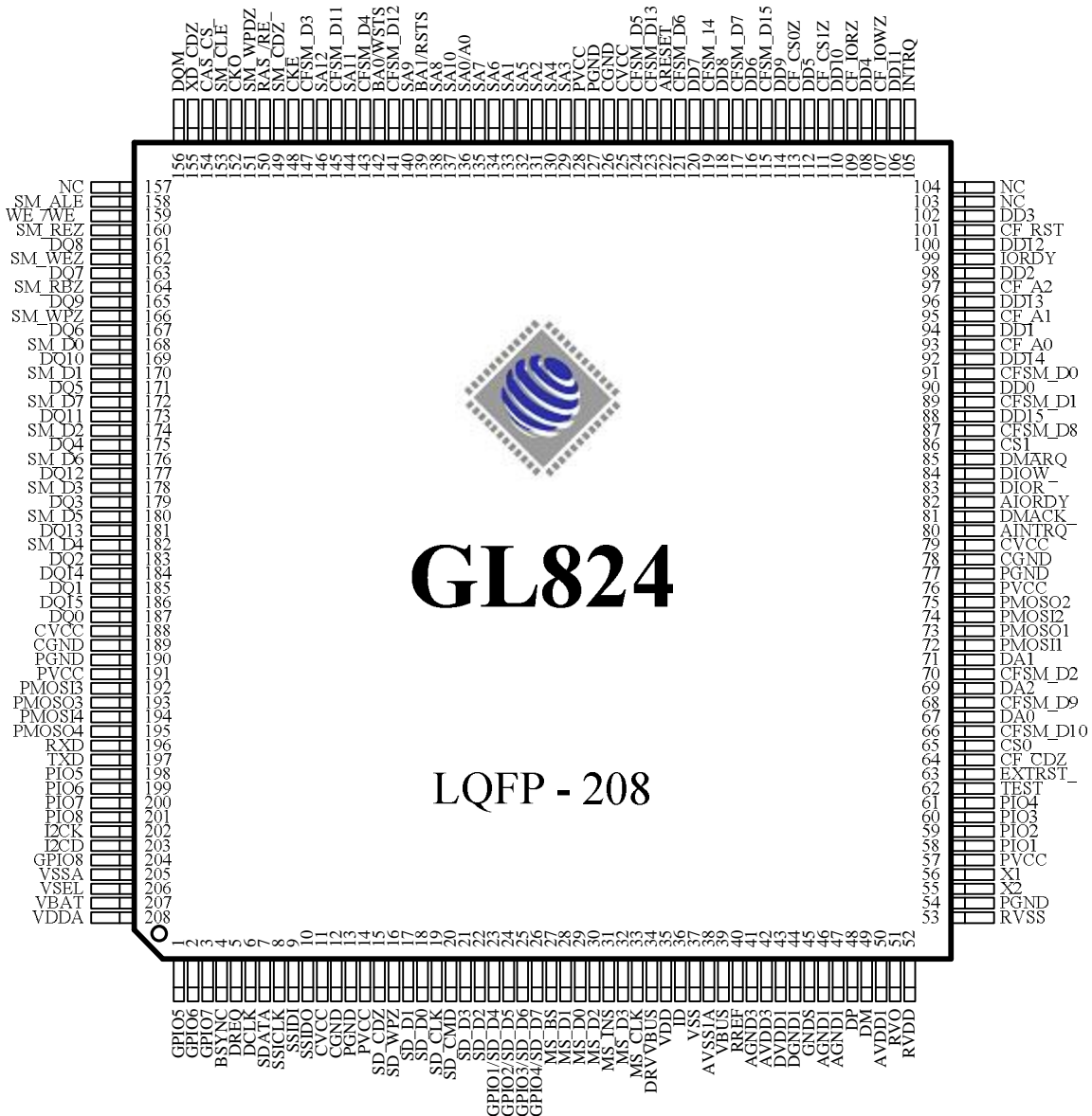
Figure 3.1 - 208 Pin LQFP Pinout Diagram
