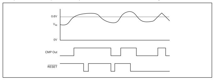
Figure 7. Comparator 1 Latching Capability
