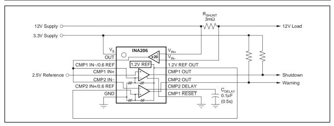
Figure 8. Server 12V Supply Current Monitor
