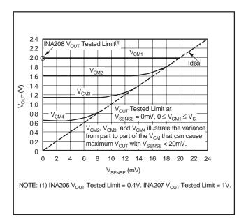
Figure 4. Example for Low V<sub>SENSE</sub> Case 2 (INA208, Gain = 100)
