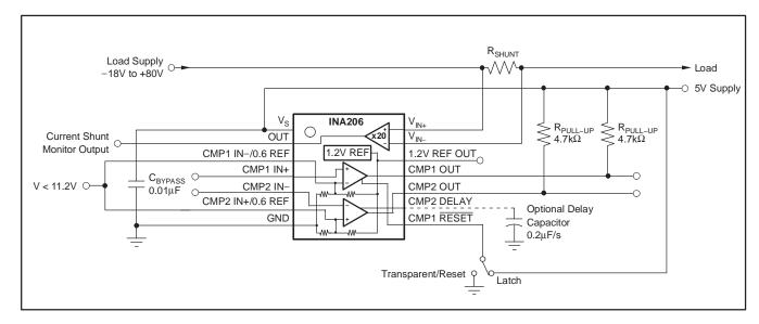
Figure 10. Overdriving Comparator Inputs Without Generating a Reference Error
