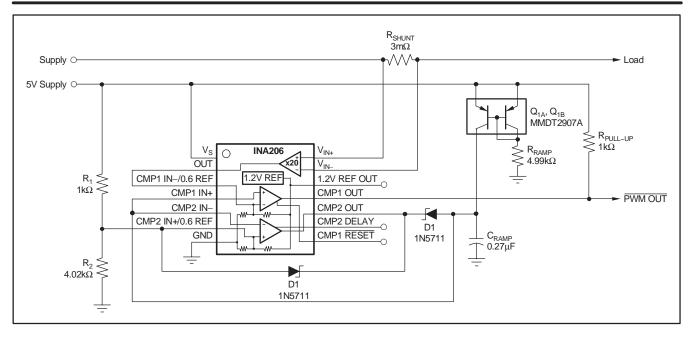
Figure 11. PWM Output Current-Shunt Monitor
