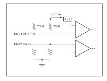
Figure 9. Limit Current Into Reference ≤ 1mA
