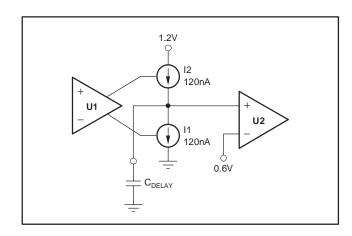
Figure 6. Simplified Model of the Comparator 2
