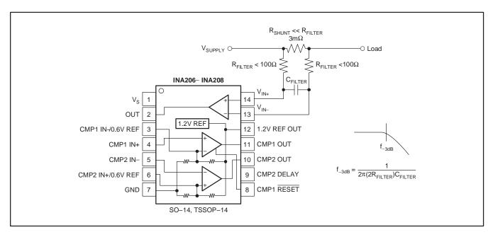
Figure 5. Input Filter (Gain Error – 1.5% to –2.2%)
