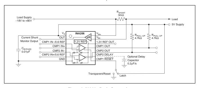
Figure 2. INA20x Basic Connection
