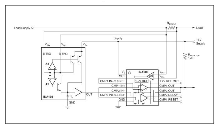
Figure 12. Bi-Directional Current Comparator
