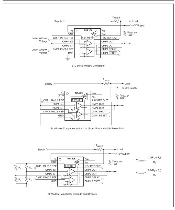
Figure 13. Using the INA206, INA207, and INA208 as Window Comparators
