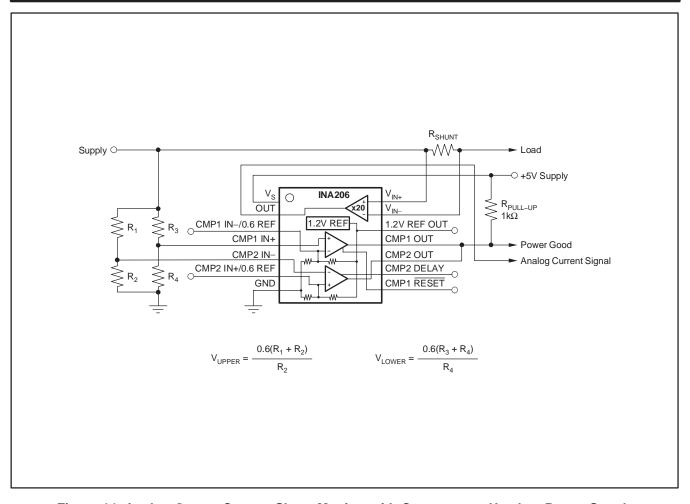
Figure 14. Analog Output Current-Shunt Monitor with Comparators Used as Power-Supply Under-Limit/Over-Limit or Power-Good Detector
