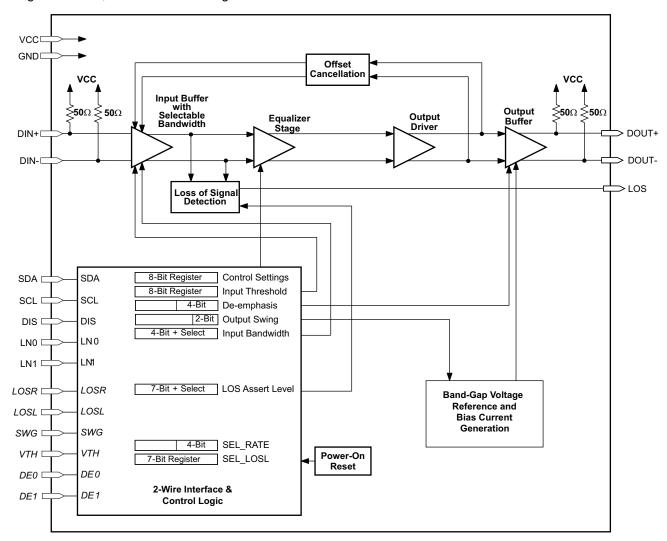
Figure 1. Simplified Block Diagram of the TLK1101E
