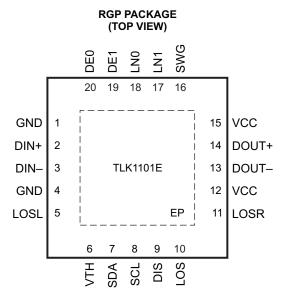
Figure 2. Pin-Out of the TLK1101E in a 4-mm  $\times$  4-mm 20-Pin QFN Package
