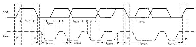
Figure 4. Two-Wire Serial Interface Timing Diagram.
