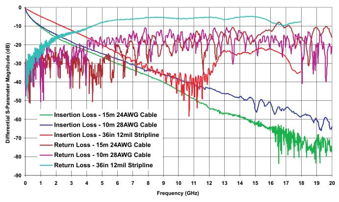
Figure 6. Typical Differential S-Parameter Characteristics of Interconnect Lines
