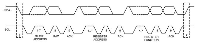
Figure 5. Two-Wire Serial Interface Data Transfer
