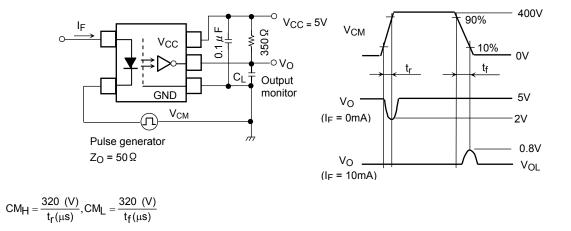
$C_L$  is approximately 15pF which includes probe and stray wiring capacitance.
