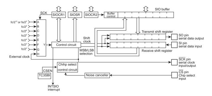
Figure 12-1 Configuration of the Serial Interface
