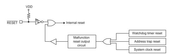
Figure 2-15 Reset Circuit
