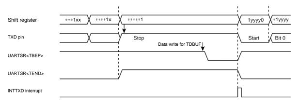
Figure 13-10 Generation of Transmit End Flag and Transmit Data Buffer Empty
