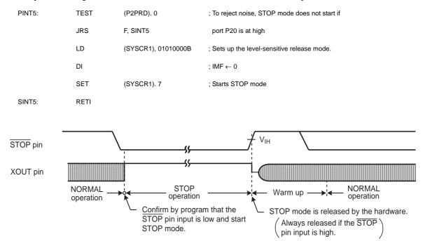
Example 2 :Starting STOP mode from NORMAL mode with an INT5 interrupt.
