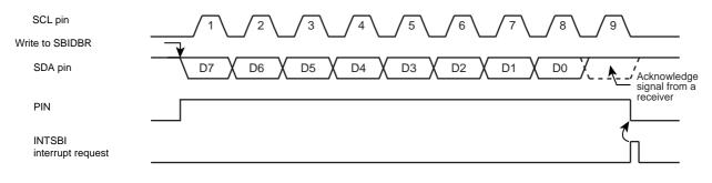
Figure 14-10 Example of when BC = "000", ACK = "1"
