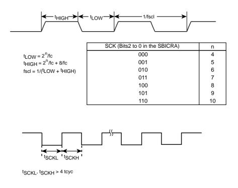
Note 1: fc = High-frequency clock Note 2: tcyc = 4/fc (in NORMAL mode, IDLE mode)
