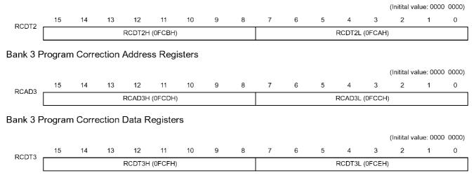
Note 1: The program correction address registers (RCADx) can only be used for specifying addresses of the user ROM area. If they are used for specifying addresses of other areas (such as SFR, RAM, and boot ROM), the address jump or data replacement mode is not enabled even though it is selected through the ROMCCR. (x: 0 to 3)
