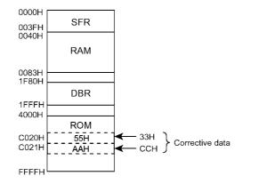
Figure 4-7 Example of Replacing the Data (2-byte data replacement mode)
