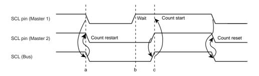
Figure 14-4 Clock Synchronization
