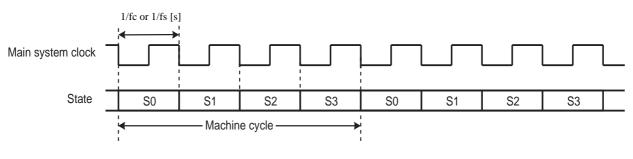
Figure 2-5 Machine Cycle
