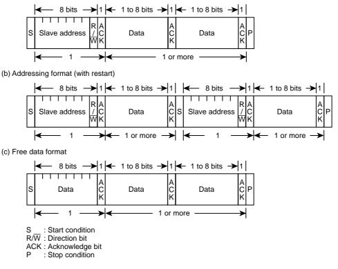
Figure 14-2 Data Format in of I<sup>2</sup>C Bus
