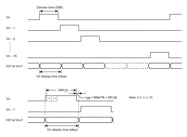
Figure 17-3 VFT Drive Wafeform and Display Timing
