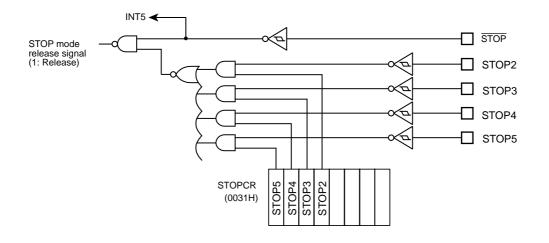
Figure 16-1 Key-on Wakeup Circuit
