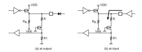
Figure 17-6 External Circuit Interface
