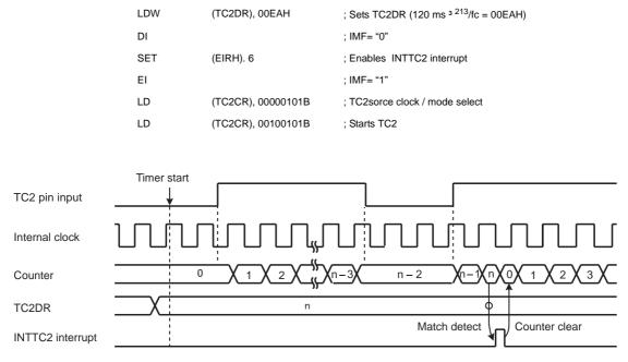
Example :Generates an interrupt, inputting "H" level pulse width of 120 ms or more. (at fc = 16 MHz, TBTCR<DV7CK> = "0")
