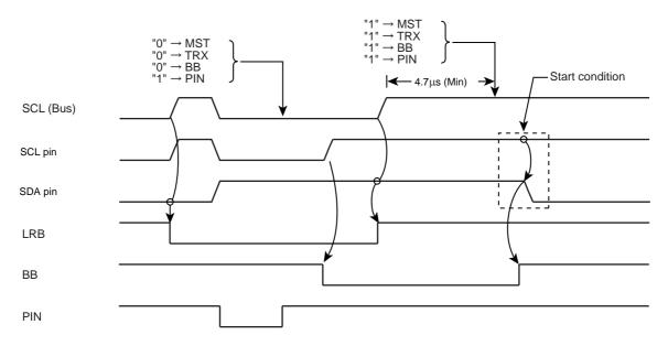
Figure 14-14 Timing Diagram when Restarting
