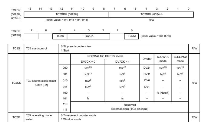
Note 1: fc: High-frequency clock [Hz], fs: Low-frequency clock [Hz], \*: Don't care
