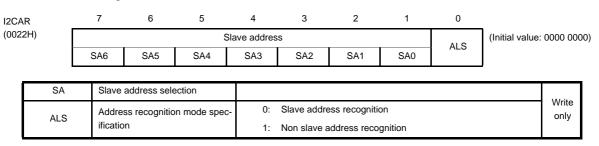
Note 1: I2CAR is write-only register, which cannot be used with any of read-modify-write instruction such as bit manipulation, etc. Note 2: Do not set I2CAR to "00H" to avoid the incorrect response of acknowledgment in slave mode. ( If "00H" is set to I2CAR as the Slave Address and a START Byte "01H" in I<sup>2</sup>C bus standard is recived, the device detects slave address match.)
