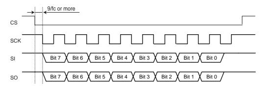
Note: The internal SCK signal goes avilable after 9/fc[s] due to the Noise-cancellation function.
