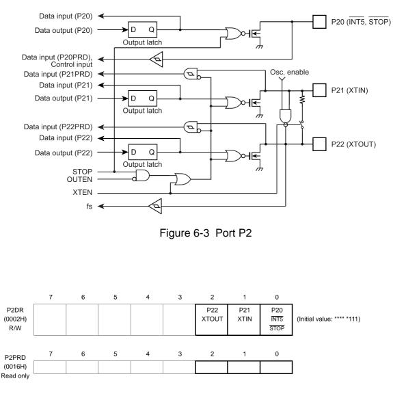
Note: Because pin P20 is used also as the STOP pin, its output high impedance becomes high when it enters the STOP mode regardless of the state of OUTEN.
