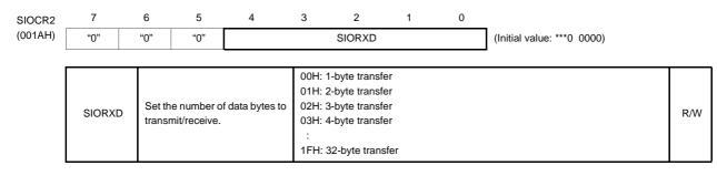
Note 1: Before setting the number of data bytes to transfer, make sure the SIO is idle (SIOSR<SIOF> = "0").
