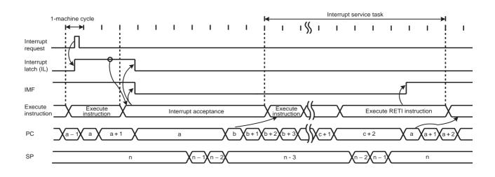
Note 1: a: Return address entry address, b: Entry address, c: Address which RETI instruction is stored Note 2: On condition that interrupt is enabled, it takes 38/fc [s] or 38/fs [s] at maximum (If the interrupt latch is set at the first machine cycle on 10 cycle instruction) to start interrupt acceptance processing since its interrupt latch is set.
