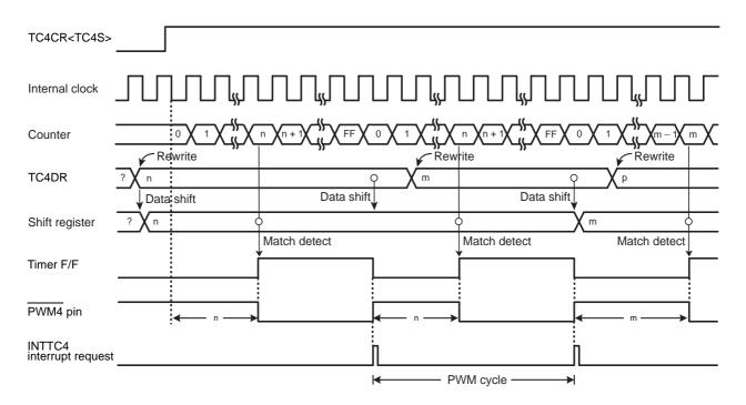
Figure 11-3 PWM output Mode Timing Chart (TC4)
