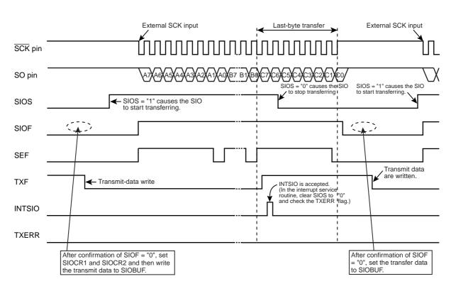
Figure 12-8 Transmit Mode Operation (where 3 bytes are transferred on an external source clock)
