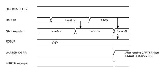
Figure 13-7 Generation of Overrun Error
