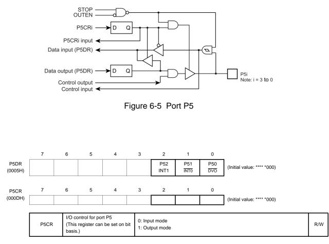
Note: If a port is in input mode, it senses the state of an input to its pins. If some pins of the port are in input mode, and others are in output mode, the content of the output latch related to a port pin that is in input mode may be changed when a bit manipulation instruction is executed on the port.
