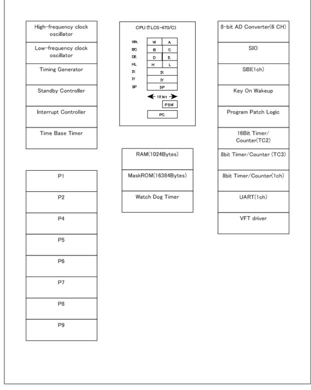
Figure 1-2 Block Diagram
