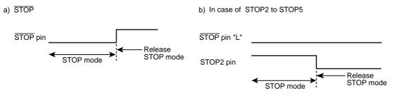
Figure 16-3 Priority of STOP pin and STOP2 to STOP5 pins
