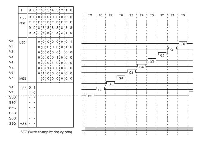
Figure 17-4 Example of Conventional type VFT driver pulse
