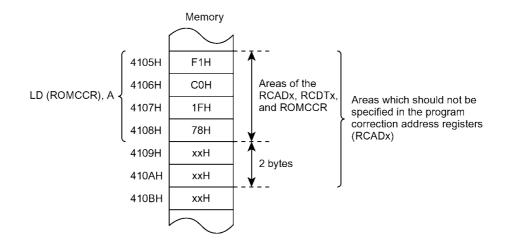
Figure 4-2 Program Correction Address Register and Data Register
