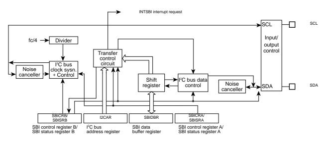
Figure 14-1 Serial Bus Interface (SBI)
