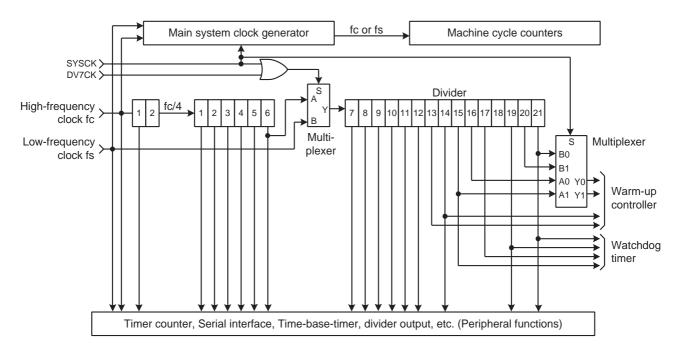
Figure 2-4 Configuration of Timing Generator
