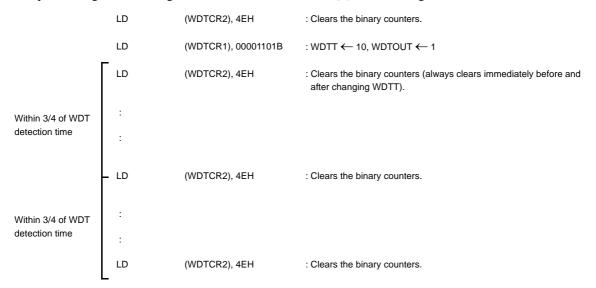
Note: The watchdog timer consists of an internal divider and a two-stage binary counter. When the clear code 4EH is written, only the binary counter is cleared, but not the internal divider. The minimum binary-counter overflow time, that depends on the timing at which the clear code (4EH) is written to the WDTCR2 register, may be 3/ 4 of the time set in WDTCR1<WDTT>. Therefore, write the clear code using a cycle shorter than 3/4 of the time set to WDTCR1<WDTT>.
