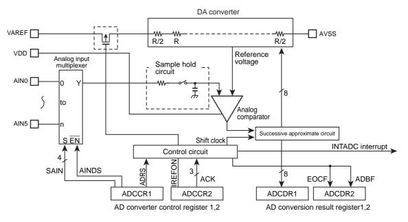
Figure 15-1 8-bit AD Converter (ADC)
