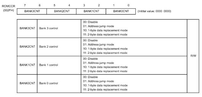
Note 1: If the BANKxCNT is set to a value other than "00B" for the bank, it is impossible to write to the program correction address registers (RCADxL, RCADxH) and program correction data registers (RCDTxL, RCDTxH) (although the write instruction is executed). Thus, a mode must be selected through the ROMCCR after all these registers are set.
