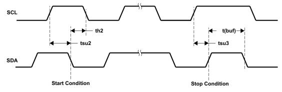
Figure 2. Start and Stop Conditions Timing
