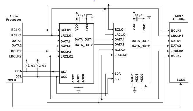
Figure 11. Two Devices Connected in Series
