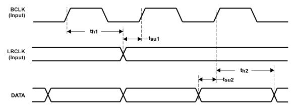
Figure 3. Serial Data Interface Timing
