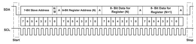
Figure 5. Typical I<sup>2</sup>C Sequence
