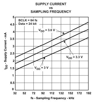
Figure 12. Typical Supply Current
