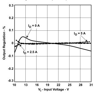
Figure 14. Output Regulation % vs. Input Voltage
