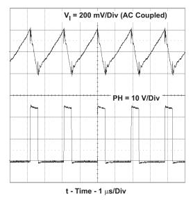
Figure 15. Input Voltage Ripple and PH Node, Io = 5 A.
