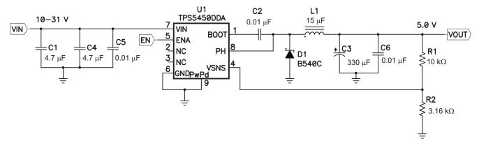
Figure 11. Application Circuit, 12-V to 5.0-V
