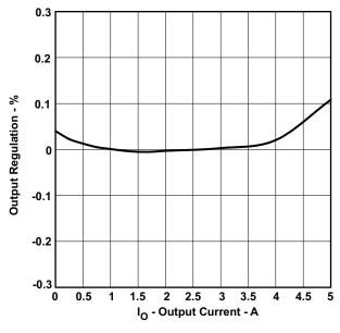
Figure 13. Output Regulation % vs. Output Current
