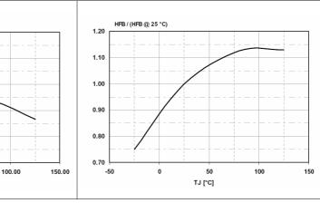
Figure 11. Brown out threshold vs T<sub>J</sub>
