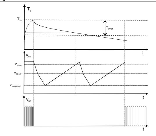
Figure 19. Thermal shutdown
