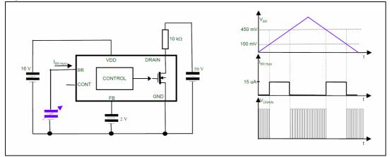
Figure 6. OVP threshold test circuits
