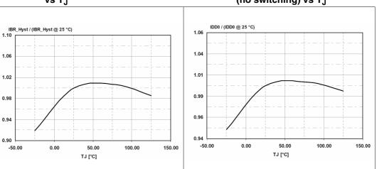
Figure 13. Brown out hysteresis current Figure 14. Operating supply current (no switching) vs T<sub>J</sub> vs T<sub>J</sub>
