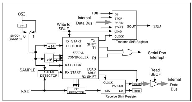
Figure 22. Serial Port Mode 2
