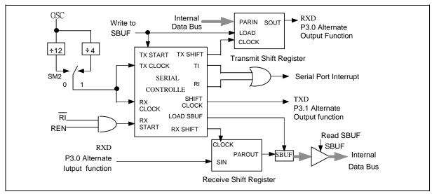
Figure 20. Serial Port Mode 0
