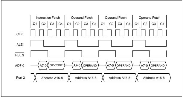
Figure 6. Four Cycle Instruction Timing
