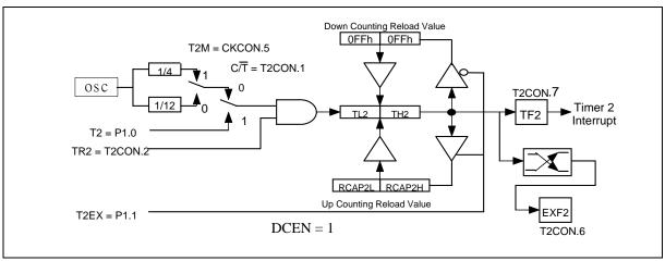
Figure 16. 16-Bit Auto-reload Up/Down Counter
