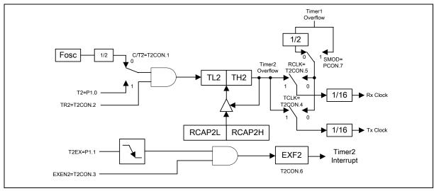
Figure 17. Baud Rate Generator Mode
