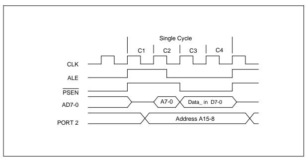
Figure 3. Single Cycle Instruction Timing
