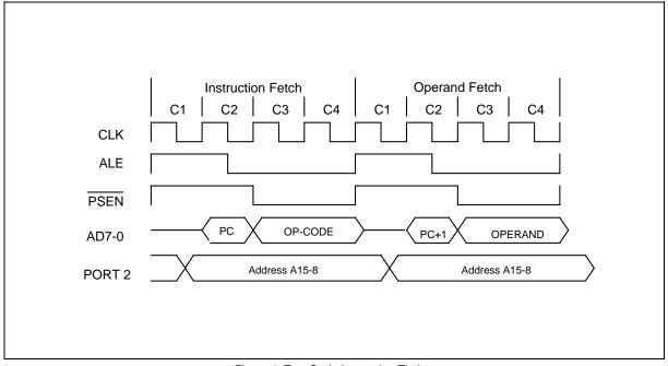
Figure 4. Two Cycle Instruction Timing
