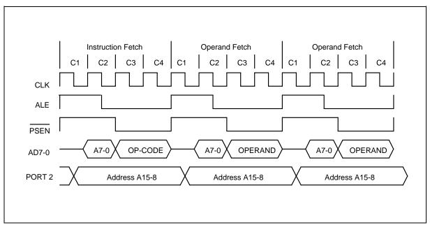
Figure 5. Three Cycle Instruction Timing
