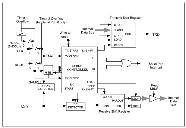
Figure 21. Serial Port Mode 1
