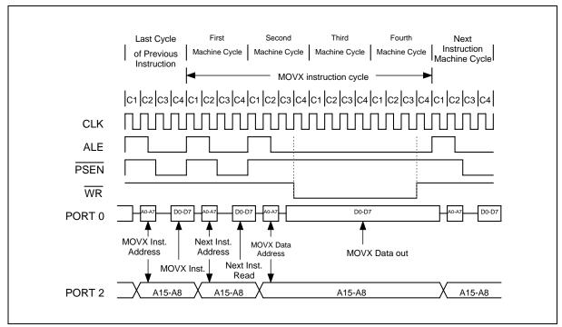
Figure 10. Data Memory Write with Stretch Value = 2
