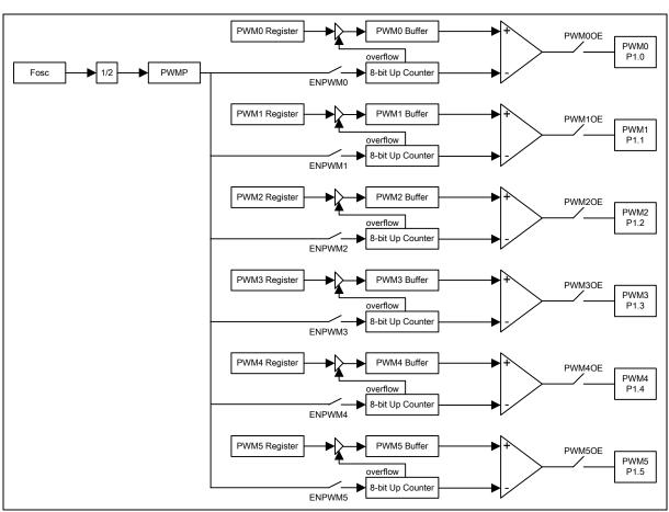
FIGURE 1 PWM DIAGRAM
