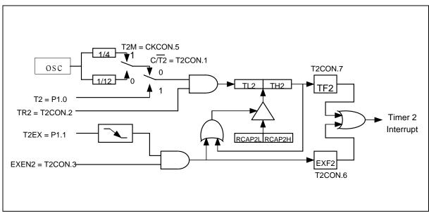
Figure 15. 16-Bit Auto-reload Mode, Counting Up
