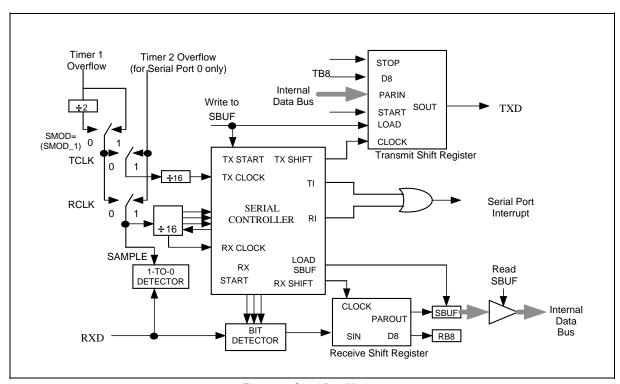
Figure 23. Serial Port Mode 3
