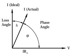
In practice the current leads the voltage by some other phase angle due to the series resistance  $R_s$ . The complement of this angle is called the loss angle and:
