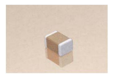
X7R formulations are called "temperature stable" ceramics and fall into EIA Class II materials. X7R is the most popular of these intermediate dielectric constant materials. Its temperature variation of capacitance is within  $\pm 15\%$  from -55°C to  $\pm 125$ °C. This capacitance change is non-linear.
