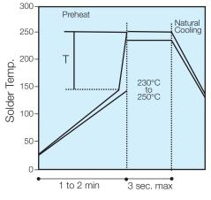
(Preheat chips before soldering) T/maximum 150°C
