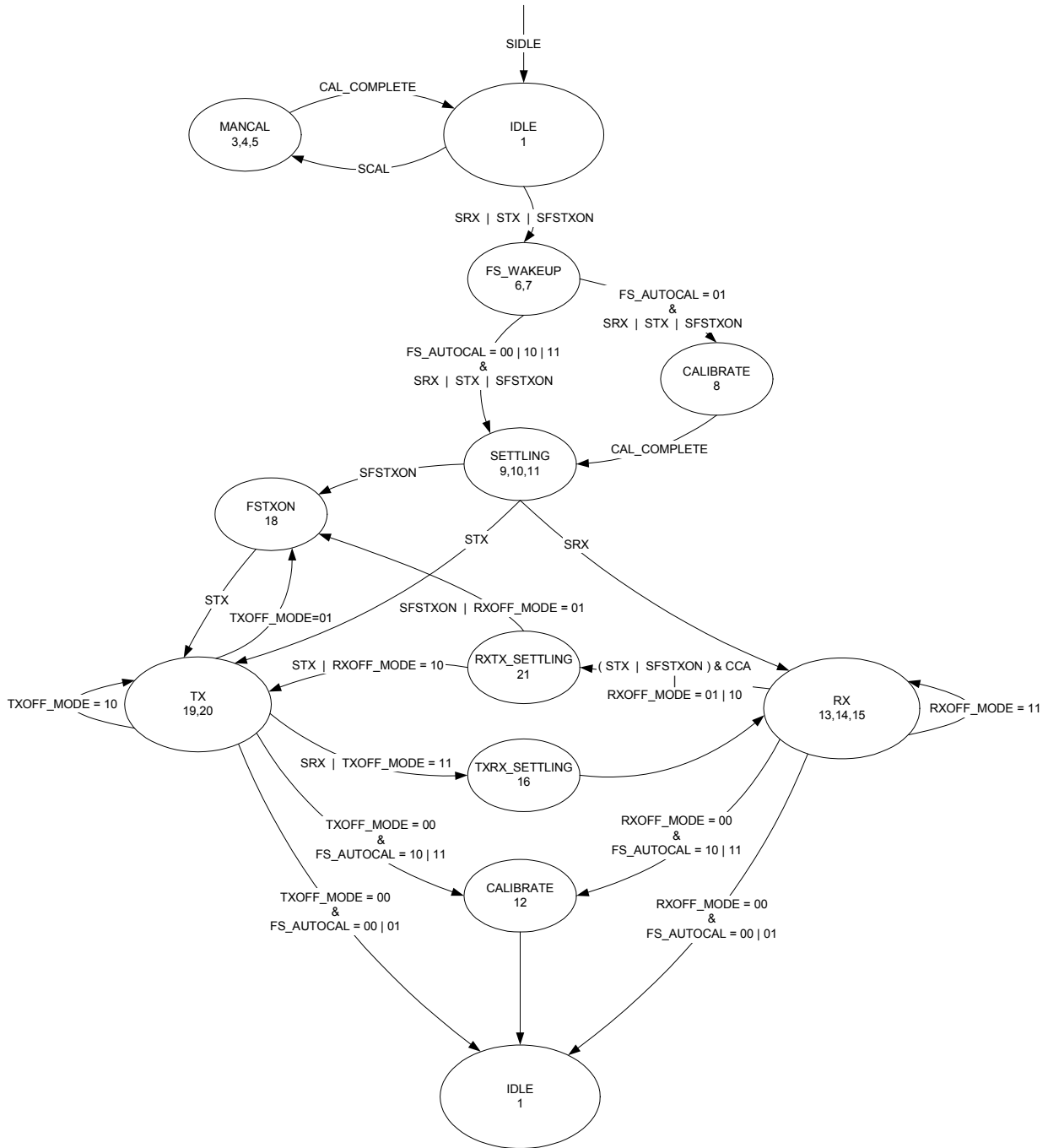
Figure 38: Complete Radio Control State Diagram
