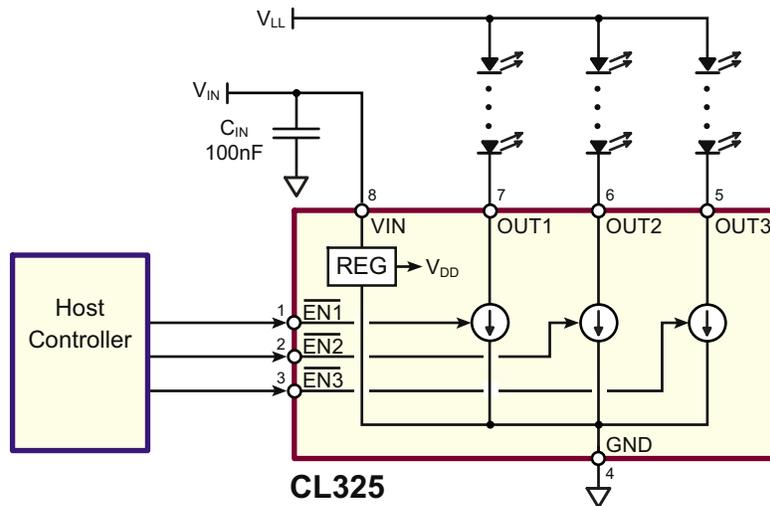
CL325 power dissipation may be lowered by supplying the CL325 from a voltage source ( $V_{IN}$ ) that is lower in voltage than the LED supply ( $V_{LL}$ ).
