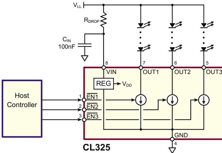
$$R_{DROP} < \frac{V_{LL(MIN)} - 6.5V}{2.3mA}$$
