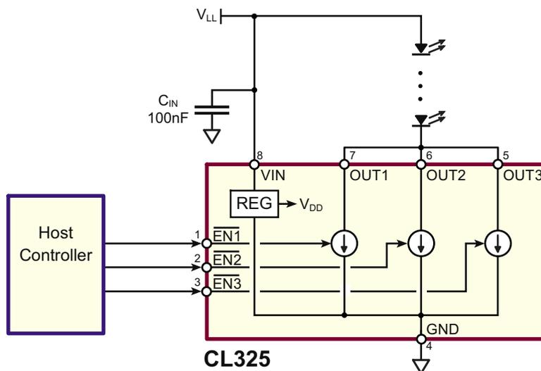
By paralleling outputs, higher LED currents can be achieved. In addition, linear dimming in 3 discrete steps may be obtained by enabling 1, 2, or 3 outputs.
