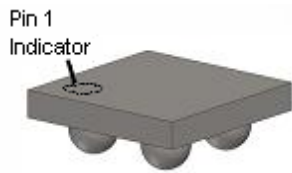
Figure 3. 1 x 1mm WLCSP Bumps Facing Down
