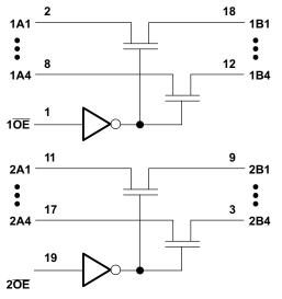
Figure 3. Simplified Schematic
