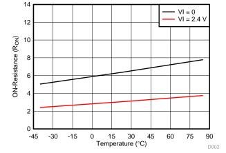
Figure 5. ON-Resistance (Ron) Variation vs Temperature
