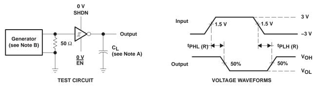
NOTES: A.  $C_{\mbox{L}}$  includes probe and jig capacitance.
