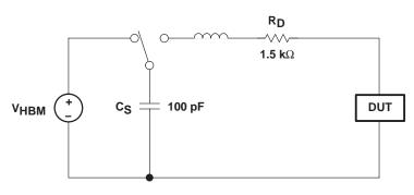
Figure 7. HBM ESD Test Circuit
