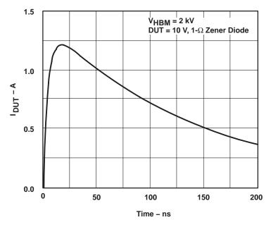
Figure 8. Typical HBM Current Waveform
