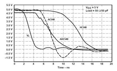
Figure 5. Switching Characteristics Comparison
