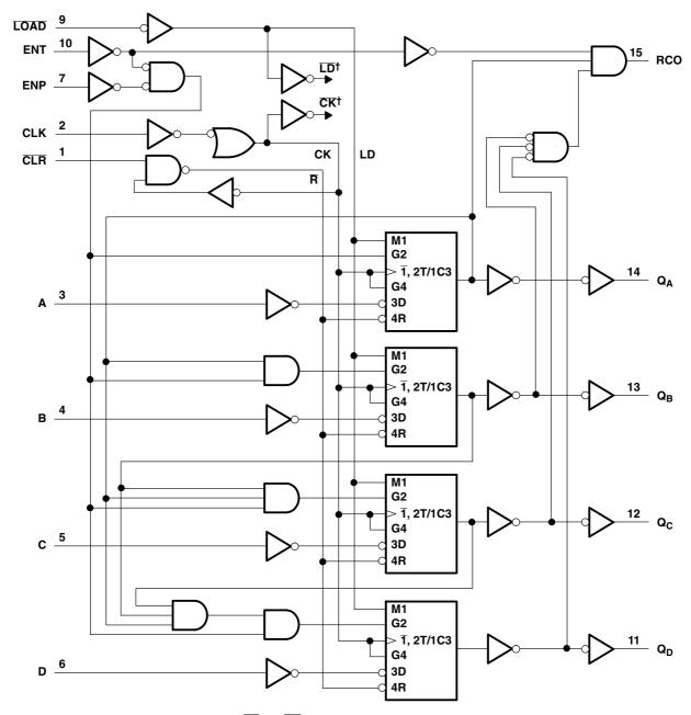
$<sup>^{\</sup>dagger}$  For simplicity, routing of complementary signals  $\overline{\text{LD}}$  and  $\overline{\text{CK}}$  is not shown on this overall logic diagram. The uses of these signals are shown on the logic diagram of the D/T flip-flops.
