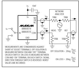
Figure 3. Off Isolation and On Loss
