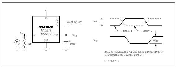
Figure 1. Charge Injection
