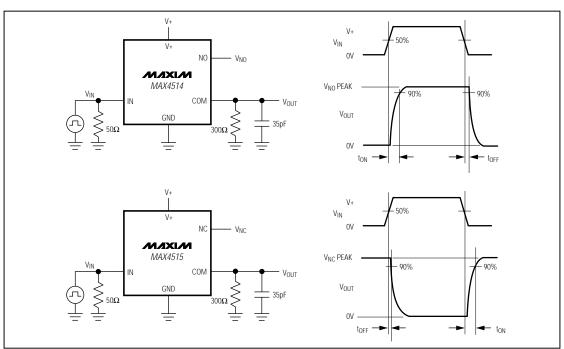
Figure 2. Switching Times
