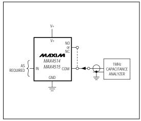
Figure 4. NO, NC, and COM Capacitance
