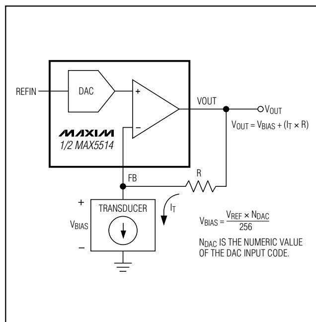
Figure 5. Transimpedance Configuration for a Voltage-Biased Current-Output Transducer
