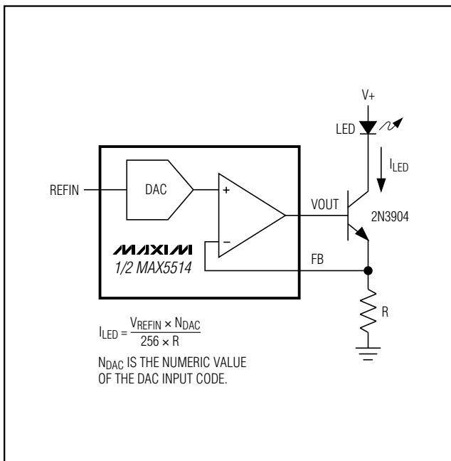
Figure 4. Programmable Current Source Driving an LED
