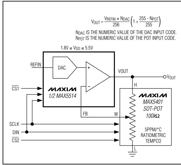
Figure 9. Software-Configurable Output Gain
