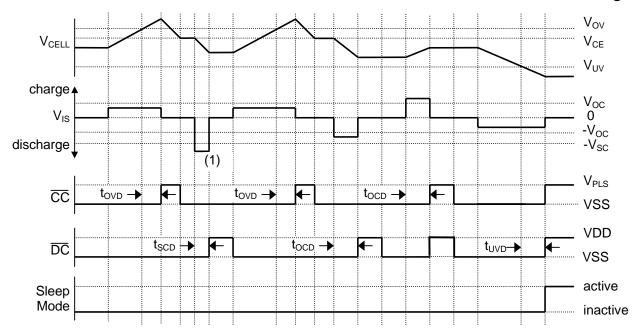
(1) To allow the device to react quickly to short circuits, detection is actually done on the SNS pin rather than on the filtered IS1 and IS2 pins. The actual short circuit detect condition is  $V_{SNS} > V_{SC}$ .
