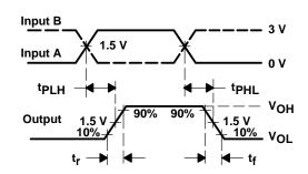
Figure 9. Receiver Switching Test Circuit and Waveforms
