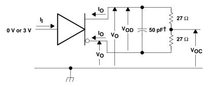
† Includes probe and jig capacitance
