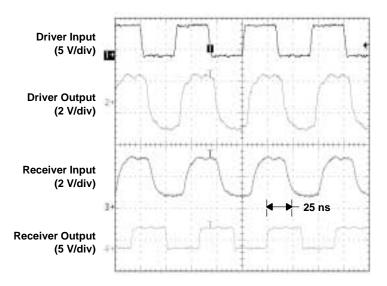
Figure 20. Signal Waveforms at 30 Mbps
