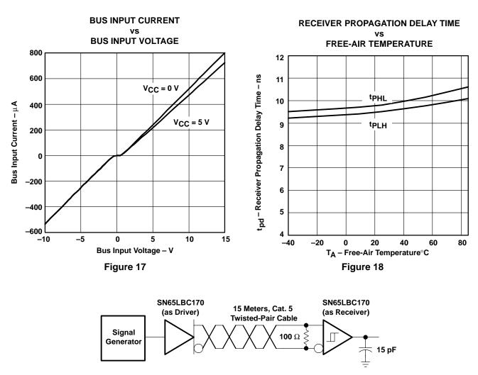
Figure 19. Circuit Diagram for Signaling Characteristics
