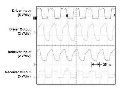
Figure 22. Signal Waveforms at 50 Mbps
