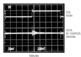
$V_{DD}$  = +5V,  $V_{SS}$  = -5V, REFAB = 2.5V,  $\overline{CS}$  = HIGH, DIN TOGGLING AT  $\frac{1}{2}$  THE CLOCK RATE, OUTA = 1.25V
