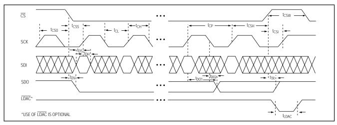
Figure 6. Detailed Serial-Interface Timing Diagram
