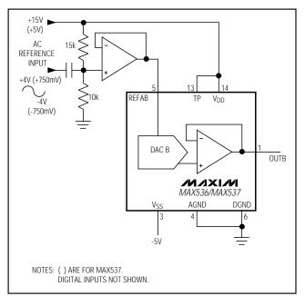
Figure 12. AC Reference Input Circuit
