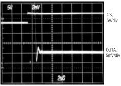
$1\mu s/div \label{eq:VDD} V_{DD}$  = +5V,  $V_{SS}$  = -5V, REFAB = 2.5V, C1 = 100pF, R1 = 10k  $\Omega$
