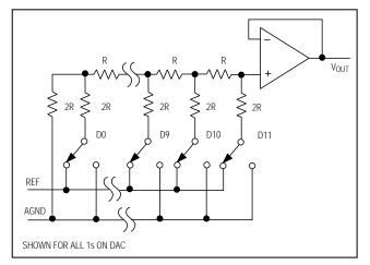
Figure 1. Simplified DAC Circuit Diagram
