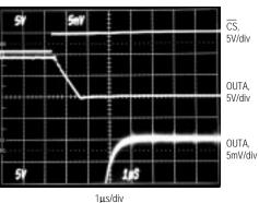
$V_{DD}$  = +15V,  $V_{SS}$  = -5V, REFAB = 10V,  $C_L$  = 100pF,  $R_L$  = 10k $\Omega$
