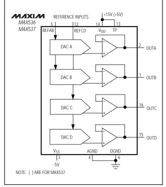
Figure 10. Unipolar Output Circuit
