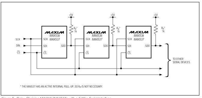
Figure 8. Daisy-Chaining MAX536/MAX537s with a 3-Wire Serial Interface
