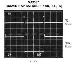
$V_{DD}$  = +5V,  $V_{SS}$  = -5V, REFAB = 2.5V,  $C_L$  = 100pF,  $R_L$  = 10k $\Omega$
