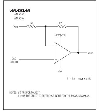
Figure 11. Bipolar Output Circuit
