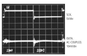
$\rm V_{DD}$  = +15V,  $\rm V_{SS}$  = -5V, REFAB = 10V,  $\overline{\rm CS}$  = HIGH, DIN TOGGLING AT  $\rm ^{1}\!\!/_{2}$  THE CLOCK RATE, OUTA = 5V
