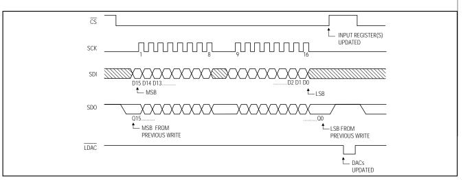
Figure 5. 4-Wire Serial-Interface Timing Diagram for Asynchronous DAC Updating Using LDAC
