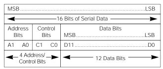
Figure 7. Serial-Data Format (MSB Sent First)
