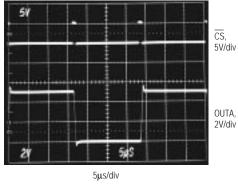
$V_{DD}$  = +15V,  $V_{SS}$  = -5V, REFAB = 5V,  $C_L$  = 100pF,  $R_L$  = 10k $\Omega$
