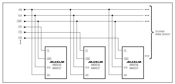
Figure 9. Multiple devices sharing a common DIN line may be simultaneously updated by bringing  $\overline{LDAC}$  low. CS1, CS2, CS3... are driven separately, thus controlling which data are written to devices 1, 2, 3...
