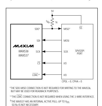
Figure 3. Connections for SPI/QSPI
