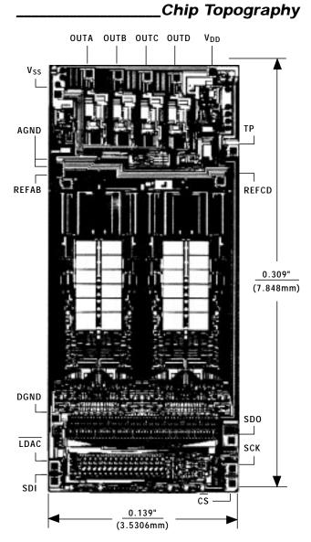
TRANSISTOR COUNT: 5034 SUBSTRATE CONNECTED TO V<sub>DD</sub>
