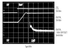
$V_{DD}$  = +15V,  $V_{SS}$  = -5V, REFAB = 10V,  $C_1$  = 100pF,  $R_1$  = 10k $\Omega$
