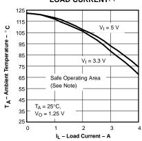
(1) Safe operating area is applicable to the test board conditions listed in the dissipation rating table section of this data sheet.
