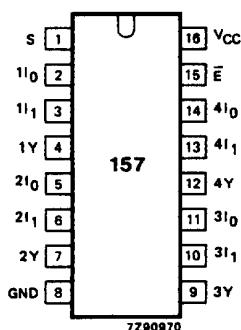
Fig.1 Pin configuration.
