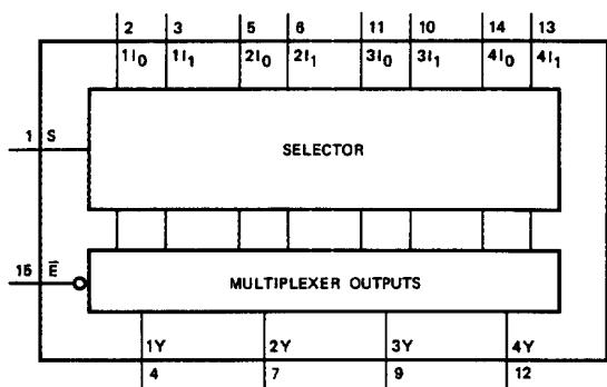
Fig.4 Functional diagram.
