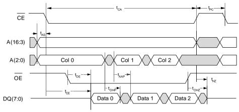
Although sequential column addressing is shown, it is not required.
