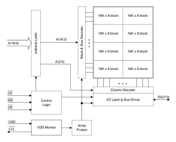
Figure 1. Block Diagram
