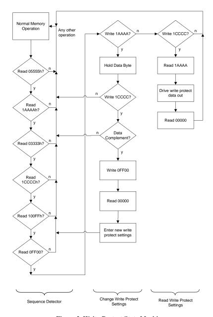
Figure 2. Write-Protect State Machine
