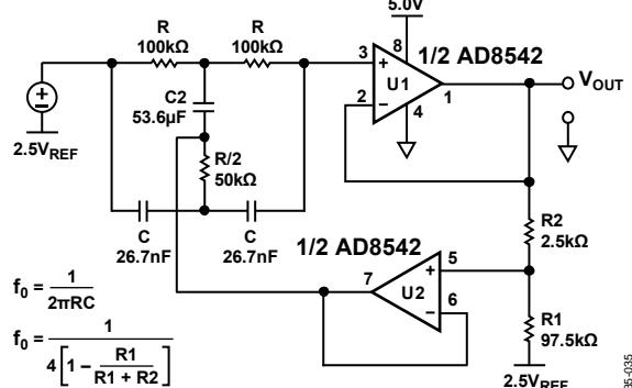
Figure 35. 60 Hz Twin-T Notch Filter,  $Q = 10$
