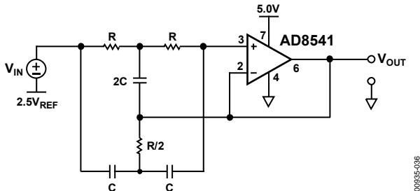
Figure 36. 60 Hz Twin-T Notch Filter,  $Q = \infty$  (Ideal)
