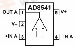
Figure 1. 5-Lead SC70 and 5-Lead SOT-23
