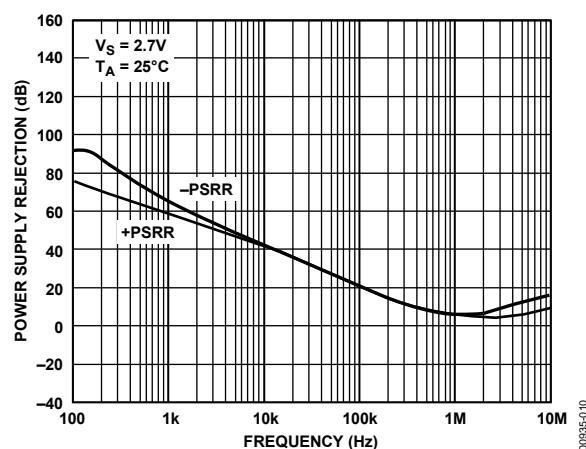
Figure 10. Power Supply Rejection Ratio vs. Frequency
