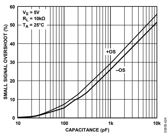
Figure 24. Small Signal Overshoot vs. Load Capacitance
