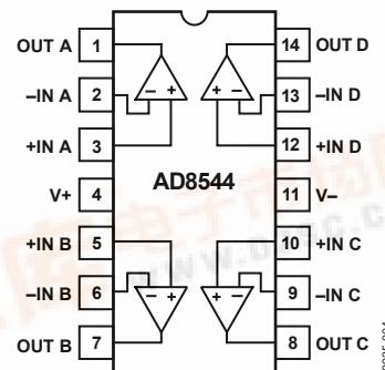
Figure 4. 14-Lead SOIC and 14-Lead TSSOP
