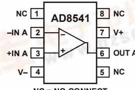
Figure 2. 8-Lead SOIC
