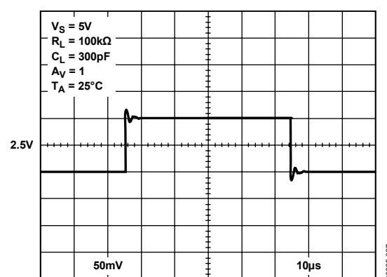
Figure 27. Small Signal Transient Response
