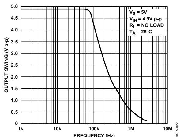
Figure 22. Closed-Loop Output Voltage Swing vs. Frequency
