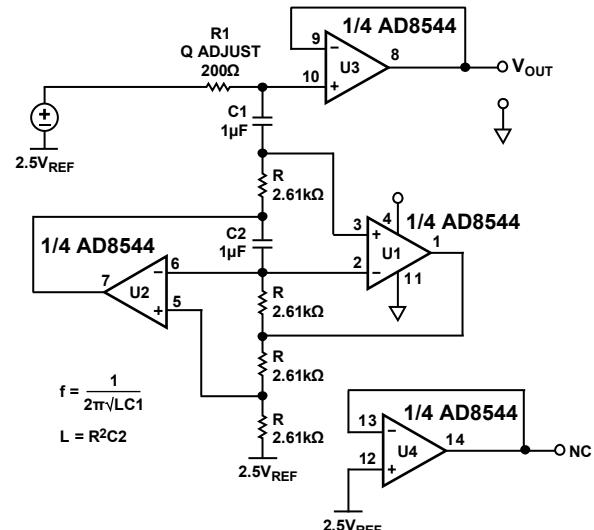
Figure 37. FNDR 60 Hz Notch Filter with Output Buffer
