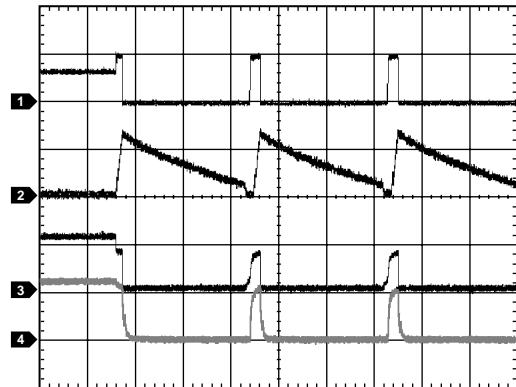
Figure 48. Overcurrent Condition During Operation (ADM1178-2 Model) (CH1 = I_{LOAD} , CH2 = V_{TIMER} , CH3 = V_{GATE} , CH4 = V_{OUT} )
