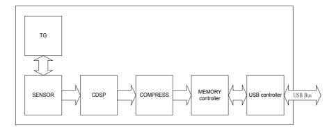
The TG block receives timing signals from the CMOS sensor and generates all the synchronization signals needed inside the SPCA561A, while the CDSP block receives and processes image data from the sensor. The image data is then further compressed by the Compression block and directly transmitted to the USB bus via the USB controller. The detailed function of each block is described in the following subsections.
