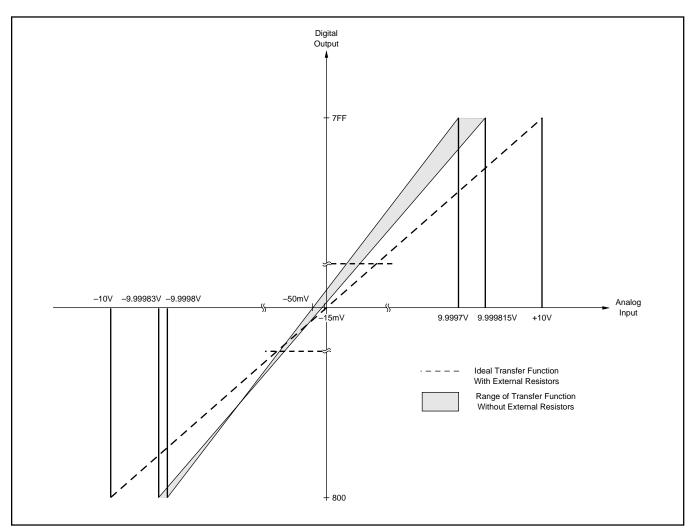
FIGURE 7. Full Scale Transfer Function.
