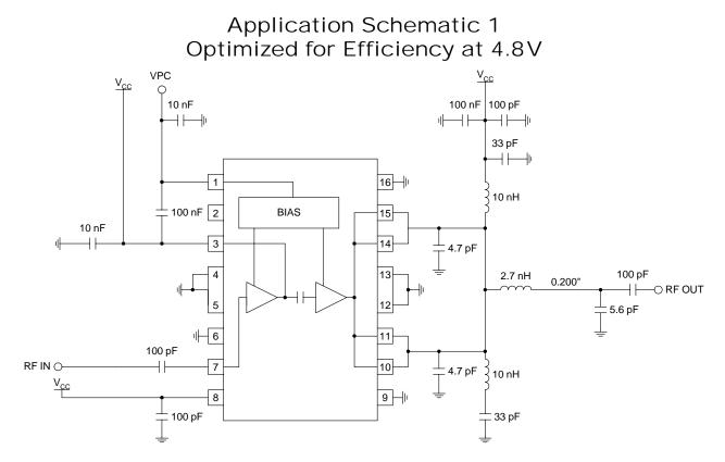
This schematic defines the optimum configuration for maximum efficiency at 4.8V. Under these conditions, as can be seen in the data plots, the power drops at 4.0V. Over 70% power-added efficiency can be achieved at +30.8dBm with 4.8V and +8dBm input level with this implementation.
