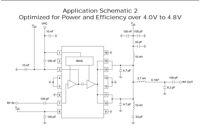
This application circuit differs from Application schematic 1 only slightly in the output tuning. The output shunt capacitor has been moved 0.060" closer to the device, and has increased from 5.6pF to 6.2pF. This retuning allows over +30.8dBm of output power to be achieved down to 4.0V, however a couple of percent points of efficiency are sacrificed. This implementation is recommended for some additional margin on output power.
