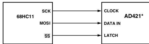
Figure 8. AD421 to 68HC11 Interface
