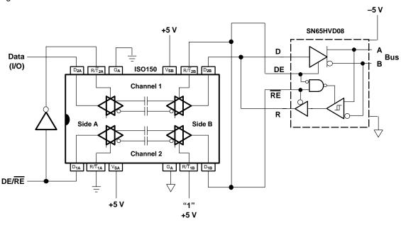
Figure 16. Isolated RS-485 Interface
