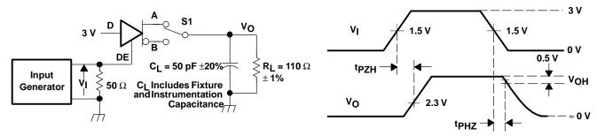
Generator: PRR = 500 kHz, 50% Duty Cycle,  $t_r$  <6 ns,  $t_f$  <6 ns,  $Z_0$  = 50  $\Omega$
