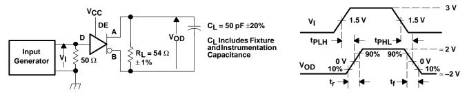
Generator: PRR = 500 kHz, 50% Duty Cycle,  $t_r$  <6 ns,  $t_f$  <6 ns,  $Z_0$  = 50  $\Omega$
