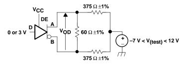
Figure 1. Driver V<sub>OD</sub> With Common-Mode Loading Test Circuit
