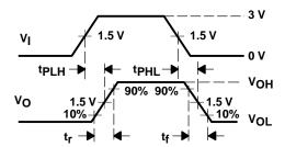
Figure 6. Receiver Switching Test Circuit and Voltage Waveforms
