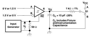
Generator: PRR = 100 kHz, 50% Duty Cycle,  $t_{\text{r}}$  <6 ns,  $t_{\text{f}}$  <6 ns,  $Z_{\text{O}}$  = 50  $\Omega$
