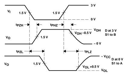
Figure 7. Receiver Enable and Disable Time Test Circuit and Voltage Waveforms With Drivers Enabled
