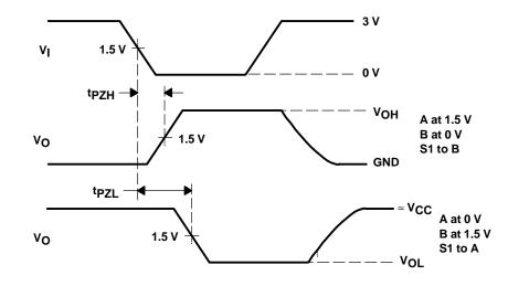
Figure 8. Receiver Enable Time From Standby (Driver Disabled)
