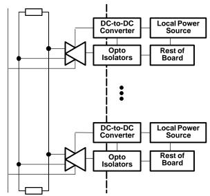
Figure 14. Isolated Power at Each Node
