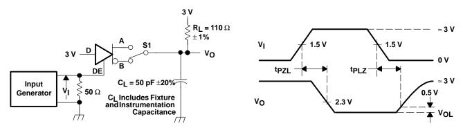
Generator: PRR = 500 kHz, 50% Duty Cycle,  $t_{\text{f}}$  <6 ns,  $t_{\text{f}}$  <6 ns,  $Z_{\text{O}}$  = 50  $\Omega$
