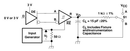
Generator: PRR = 500 kHz, 50% Duty Cycle,  $t_{f}$  <6 ns,  $t_{f}$  <6 ns,  $Z_{0}$  = 50  $\Omega$
