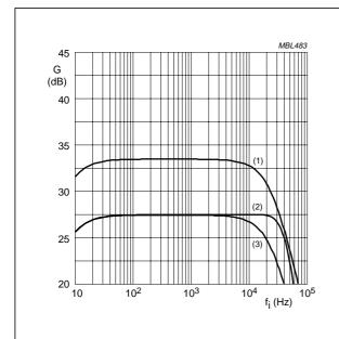
$V_P = \pm 25 \text{ V}; V_i = 100 \text{ mV}; R_s = 10 \text{ k}\Omega; C_i = 330 \text{ pF}.$
