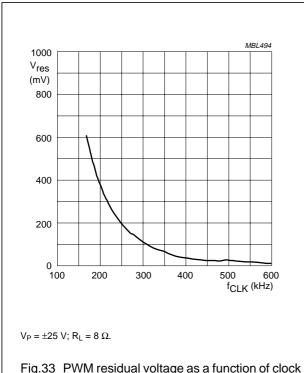
Fig.33 PWM residual voltage as a function of clock frequency.
