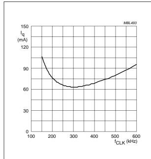
$V_P = \pm 25 \text{ V}$ ;  $R_L$  is open-circuit.
