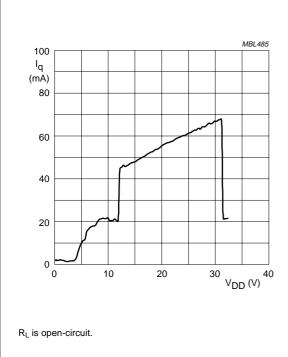
Fig.25 Quiescent current as a function of supply voltage.
