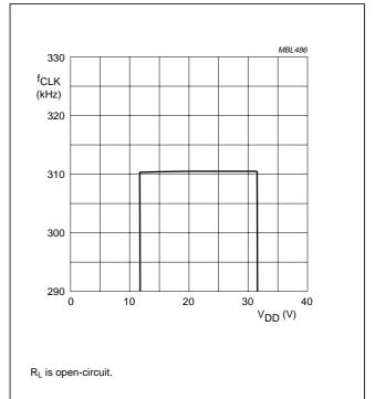
Fig.26 Clock frequency as a function of supply voltage.
