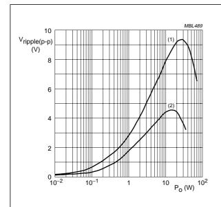
$V_P=\pm 25~V;\,3000~\mu F$  per supply line; f = 10 Hz.
