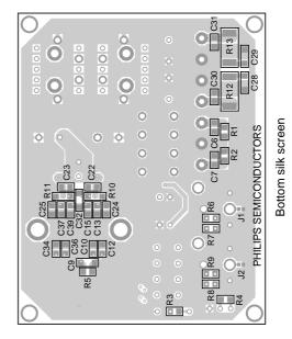
Fig.10 Printed-circuit board layout for the TDA8920TH.
