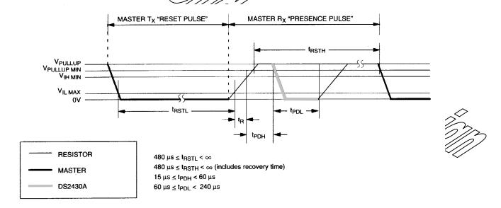
In order not to mask interrupt signaling by other devices on the 1-Wire bus,  $t_{RSTL} + t_R$  should always be less than 960 $\mu$ s.
