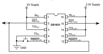
NOTE: The  $\overline{\text{RST}}_{5V}$  output is connected to the  $\text{IN}_{3.3V}$  via a 100 k $\Omega$  resistor in the push-button input and therefore does not require a pull-up resistor (an addition pull up can be used to accelerate responses). If an external pull up is used in this example it must be connected to the 3.3V power supply.
