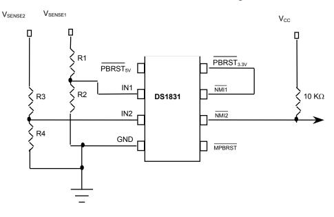
Example:  $V_{\text{SENSE1}} = 11.50 \text{V}$  trip point  $V_{\text{SENSE1}} = \frac{R1 + R2}{R2}$  X 1.25V
