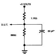
\*INCLUDING SCOPE AND JIG CAPACITANCE
