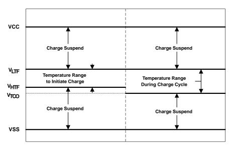
Figure 4. Temperature Sense Input Thresholds
