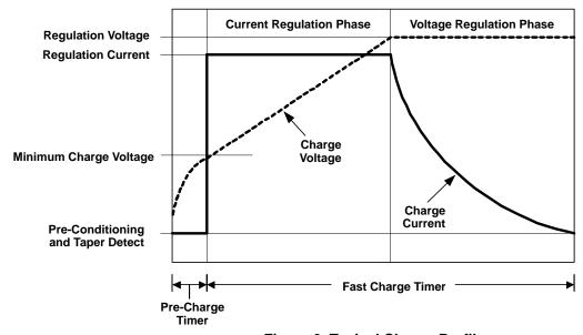
Figure 2. Typical Charge Profile
