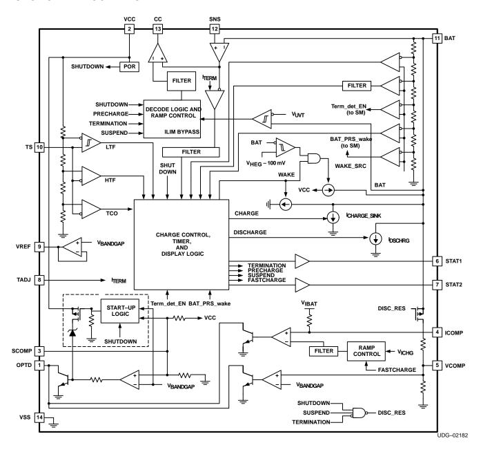
The bq24901 supports a precision current and voltage regulated li-ion charging system suitable for single-cells. Figure 1 shows the typical application diagram, Figure 2 shows a typical charge profile, and Figure 3 shows an operational flow chart.
