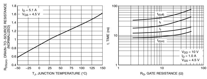
Figure 1. On–Resistance Variation with Temperature
