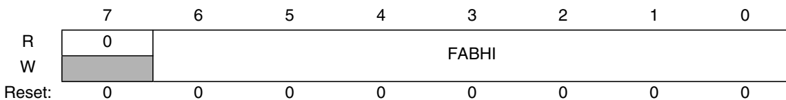
Figure 2-11. Flash Address High Register (FADDRHI)
