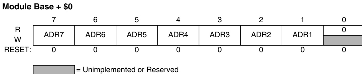
Figure 10-2. IIC Bus Address Register (IBAD)
