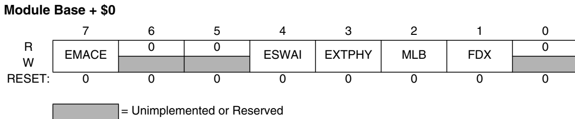
Figure 11-2. Network Control (NETCTL)
