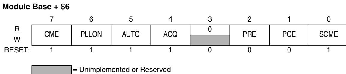
Figure 4-9. CRG PLL Control Register (PLLCTL)
